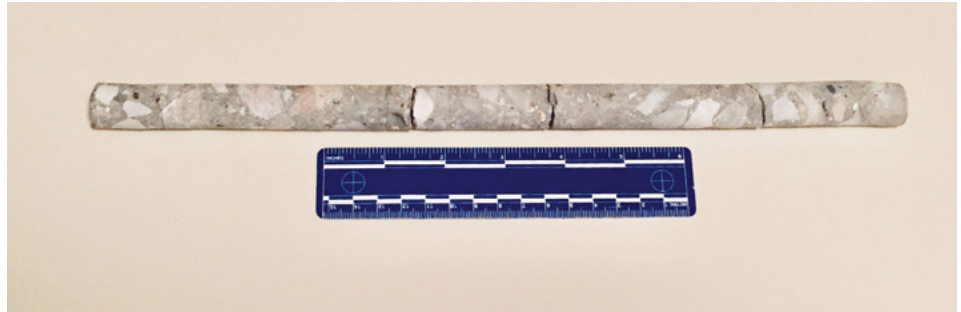
Fig 5. Half inch diameter probes used to assess integrity of interior concrete in congested members.
