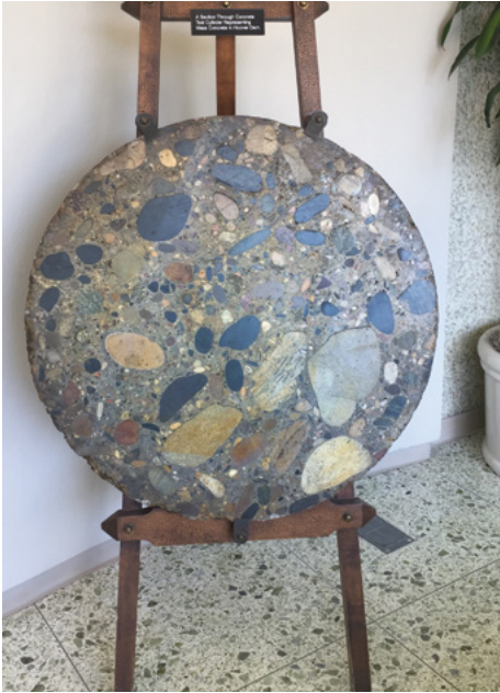
Fig. 2 Concrete core taken from the Hoover Dam constructed between 1931 and 1936.
